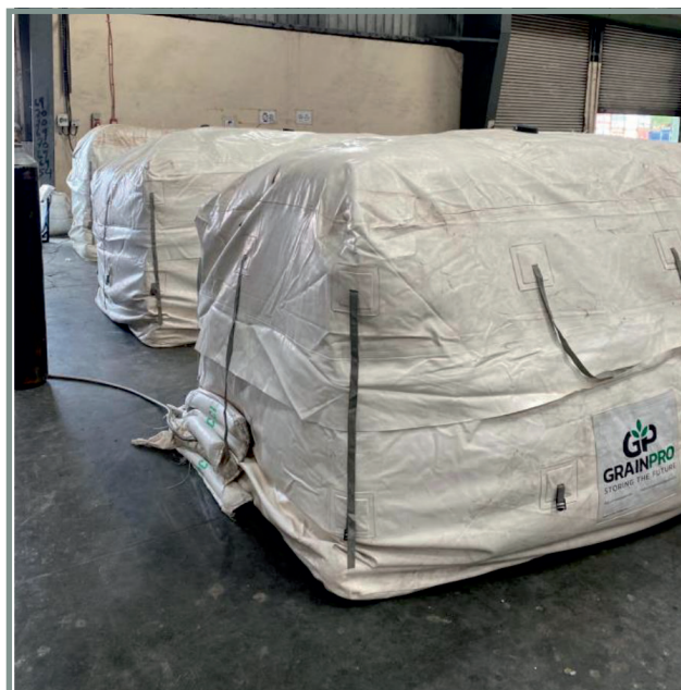
stored food grain insect management using e-fume (83.3% CO 2 + 16.7% ethyl formate) by fumigating wheat grain stacks at Jaipur.
